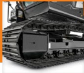
■ With large idlers, rollers and strutted track links, the sealed and lubricated undercarriage is built for the long haul.
