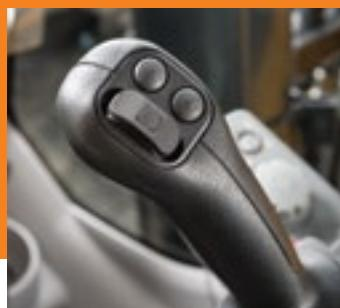
■ Ergonomically correct short-throw pilot levers provide smooth, precise control with less effort. Standard sliding switch provides proportional speed control, giving you full command from your fingertips.
